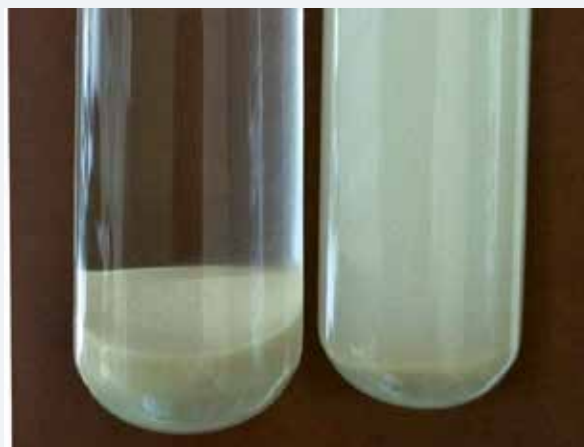
Solubilisation of MannoRelease. The combined product has been prepared in a tartrate buffer (pH 3.5) and incubated for 48 h at 25 °C
