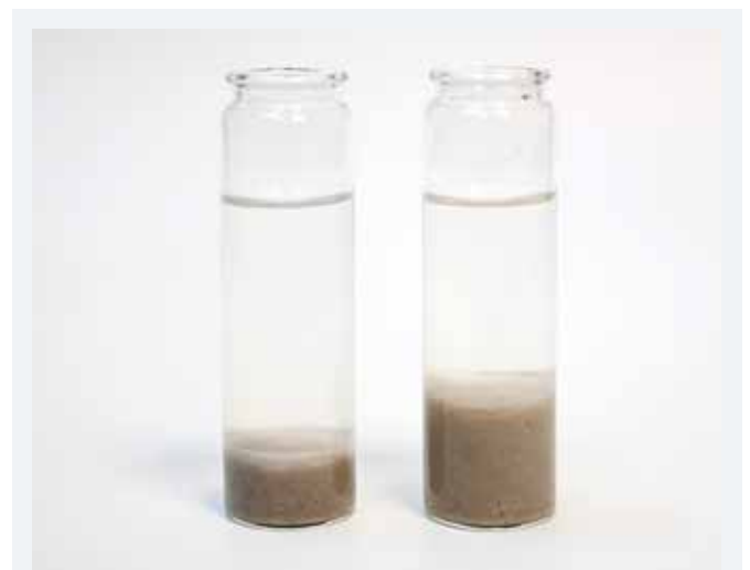
Different priming behaviour of NaCalit® PORE-TEC (left) and GranuBent® PORE-TEC (right)
